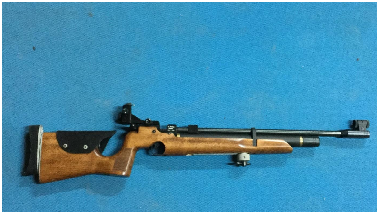
An Air Arms S200 10 metre air rifle modified with: shortened stock, adjustable butt plate, raised cheek piece and gadget rail which holds the handstop with sling loop for the sling hook. (A friendly DT teacher is invaluable for this!)
